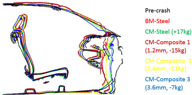
Figure 9 – Right Oblique Intrusion- Baseline vs. CM-Steel and CM-Composite
