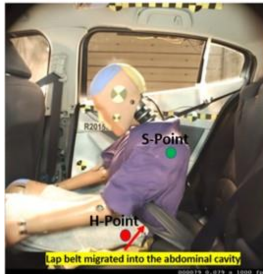
Figure 13. Unfavorable kinematics with submarining.
