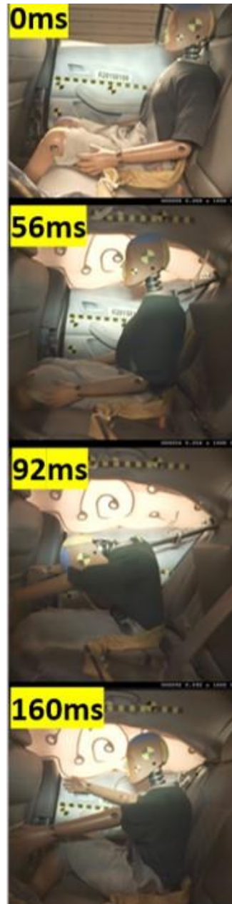
Figure 3. ATD kinematics with no submarining.
